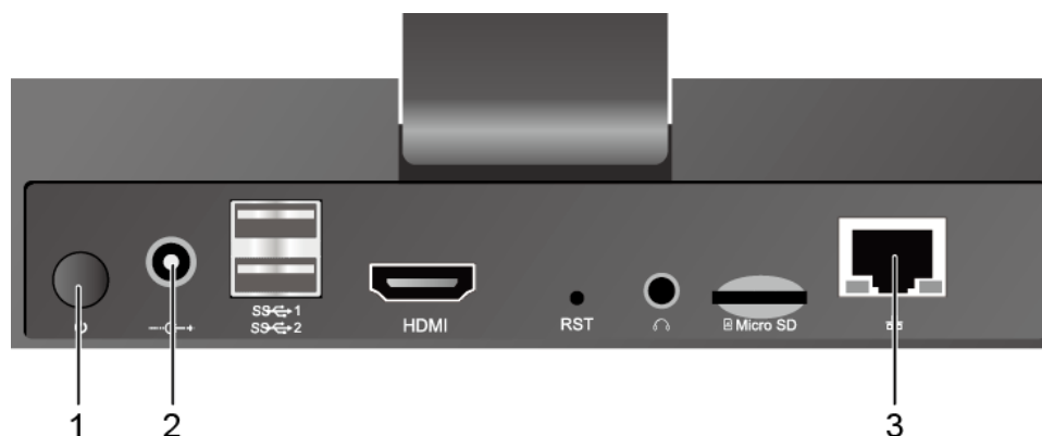
Figure 5-3 Ports on the rear panel
